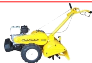
GARDEN TILLER WITH HONDA GX160 ENGINE
